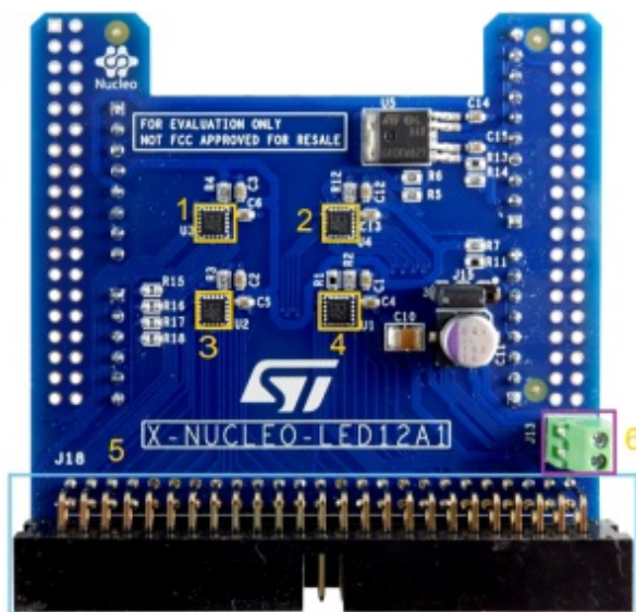
Figure 3. X-NUCLEO-LED12A1 expansion board component placement
