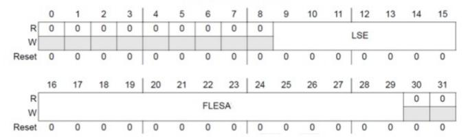
To configure the RAM area to store extended filters it is necessary to program the following values in the FLESA and LSE fields.
