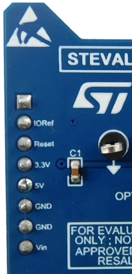
Figure 2. CN1 connector for 3.3V power supply
