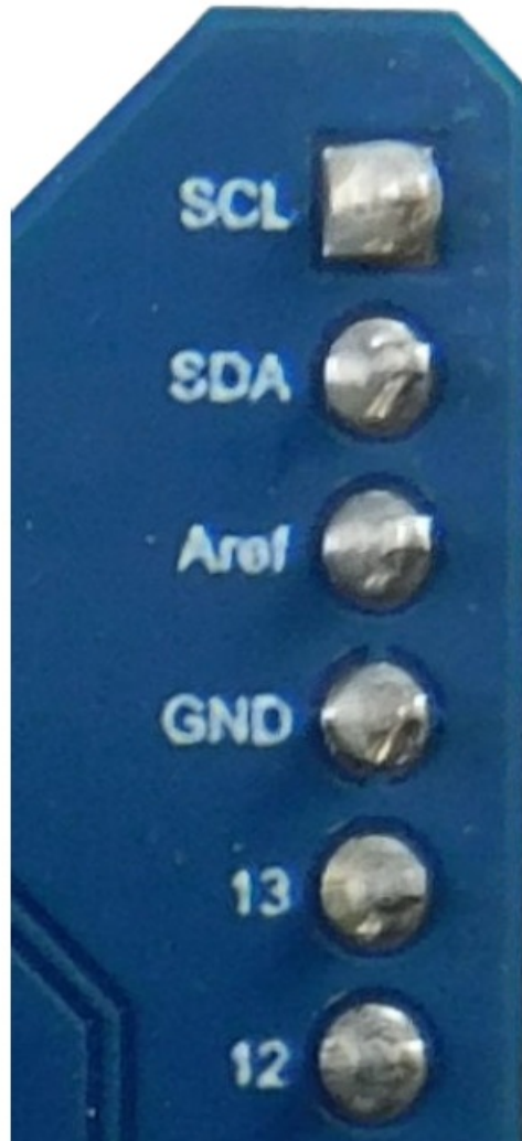
Figure 3. CN2 connector for I 2 C/I 3 C connection
