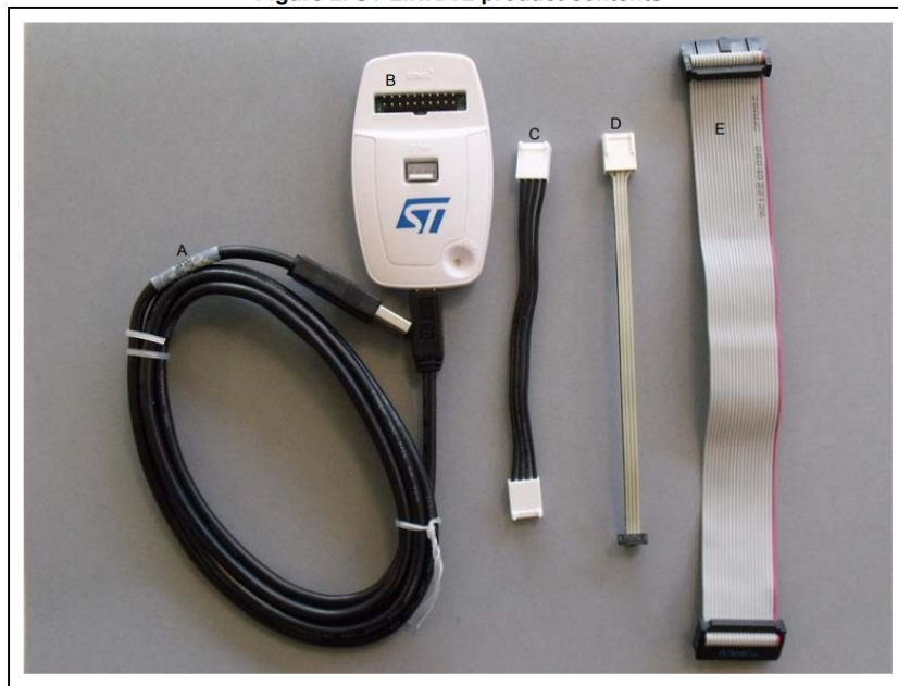
Figure 2. ST-LINK/V2 product contents
