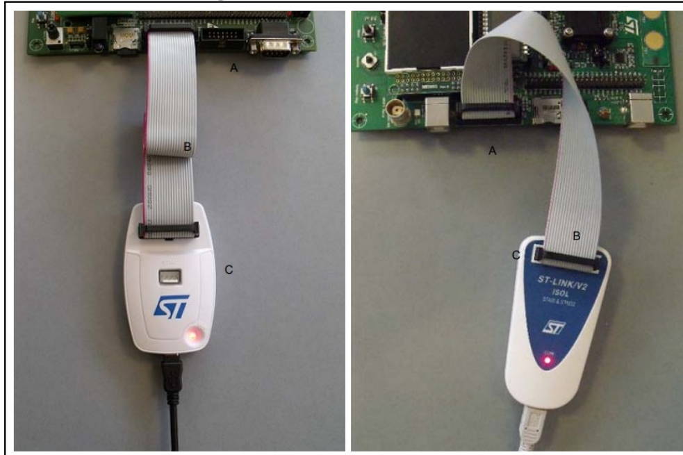
Figure 9. JTAG and SWD connection
