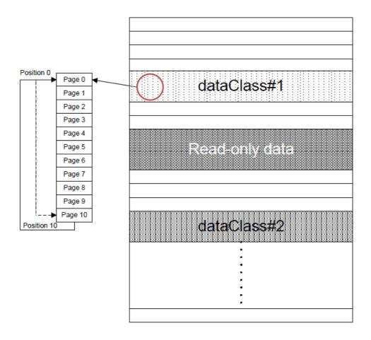
The cycle begins at pointer position 0. Each cycle, the pointer is incremented to write the next page. When the last page is reached, the position is reset. So, the 11 pages are cycled 478182 times. This strategy has the benefit of distributing the cycling over several locations and avoid max stress on a same area.
