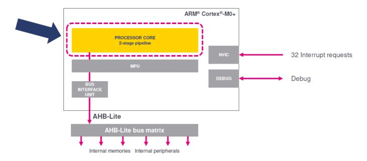
The Cortex®-M0+ core delivers more performance than the Cortex®-M0 core thanks to the 2-stage instruction pipeline.
