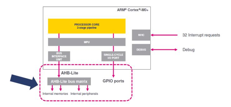
The Cortex®-M0+ has neither an embedded cache nor internal RAM. Consequently, any instruction fetch transaction is steered to the AHB-Lite interface and any data access is steered either to the AHB-Lite interface or the Single-cycle I/O port.
