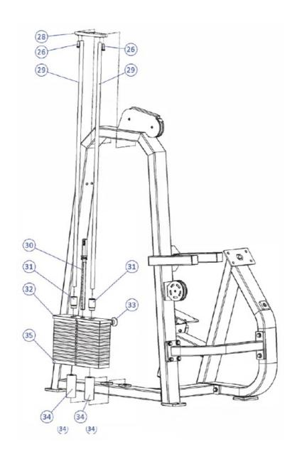
STEP 3: INSTALL ARM PAD TO MOUNTING TUBE ASSEMBLY, BOOM HANDLE ASSEMBLY. AFTER INSTALLING THE CAM(4) AND ADJUSTABLE BICEP/TRICE GRIP HANDLES, INSTALL WEIGHT PLATE CABLE STARTING AT MOUNTING LOCATION ON THE CAM(4).
