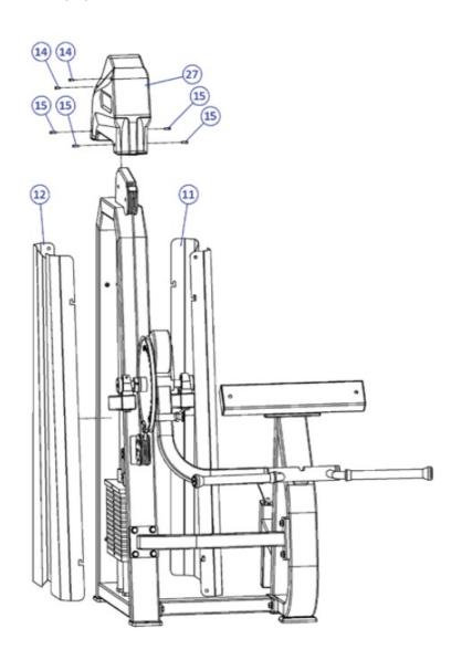
**STEP 5:** INSTALL ELBOW PADS AND SEAT CUSHIONS.
