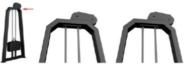
FIRST NOVE THE PLASTIC FIXING PLATE TO THE POSITION SHOWN IN THE FIGURE, AND THEN TIGHTEN IT WITH SCREWS
