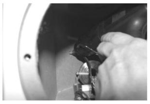
7. Pull the tweeter cable through the hole in the cabinet bracing.
