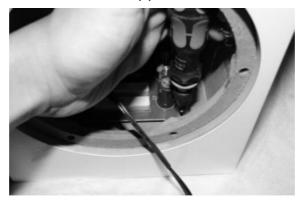
5. Pass the input wire through the hole in the rear panel of the cabinet.
