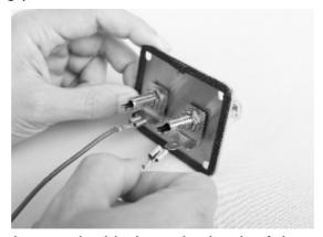
9. Mount the terminal plate to the terminal hole at the back of the cabinet.
