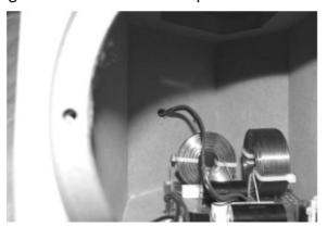
6. Seal the cable hole with hot melt glue.
