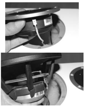
11. Carefully place the drivers in the cabinet and fasten the screws.
