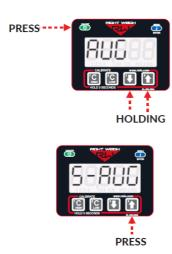
2. Press the UP arrow button to cycle through the operating modes. To confirm your selection, turn the scale off by pressing the ON/OFF button.
