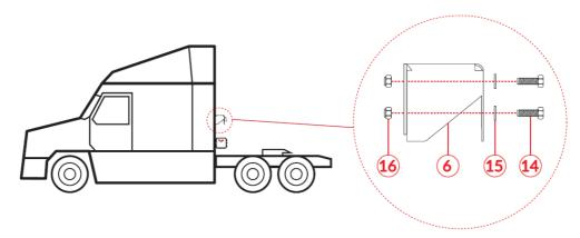
Once the mounting bracket is secure on the truck, mount the data communication socket to the bracket using the supplied hardware. Don't forget to place the Gasket between the Data Communication Socket and the Mounting Bracket.
