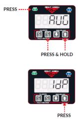
2. Press the UP arrow to change the mode to IDP. Turn off the scale to save your selection. IDP mode will measure both air sensors on the Remote Sensor separately when connected to 2 axle groups.
