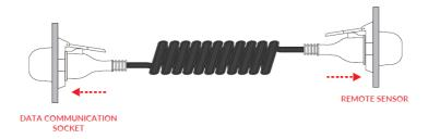
This Coiled Jumper Cable can connect to any Remote Sensor on any trailer and display a trailer weight. Each Remote Sensor will need to be connected to a tractor scale and calibrated with an empty and loaded weight before use.
