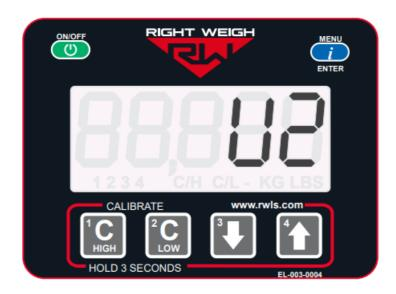
The gauge should be set to detect 2 Spring Sensors. See Spring Suspension Gauge manual for more information on how to set the sensor configuration.
