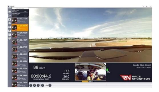
The Video Player view allows for displaying recorded movies. You can select the lap you wish to display in the Laps list, on the left side of the screen. The Laps list is displayed on the left side next to the menu column.
