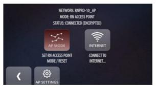
2. On the PC, click on the Wi-Fi icon on the taskbar and **connect to the proper network (device name AP).**After these steps, the Race Navigator device will be available in the **Download dialog view.**
