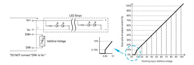
Applying additive 10V PWM signal (frequency range 100Hz ~ 3KHz)
