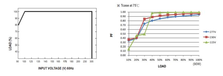
• De-rating is needed under low input voltage.
