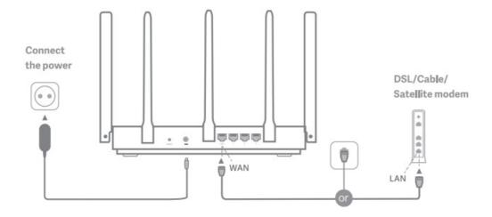
Power on the router, then connect the Internet (WAN) port to the DSL/Cable/satellite modem
