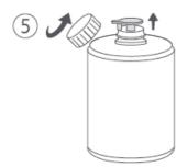
Unscrew the hand soap cover counterclockwise, and remove the silicon plug.
