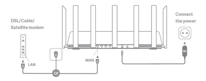
Power on the router, then connect the Internet (WAN) port to the DSL/Cable/satellite modem
