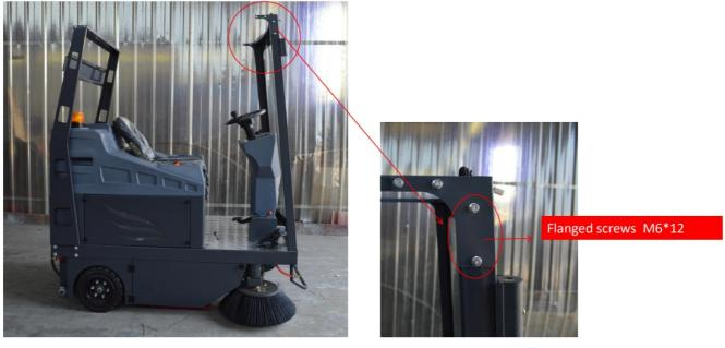
• STEP 6 Install the ceiling fixing pipe.
