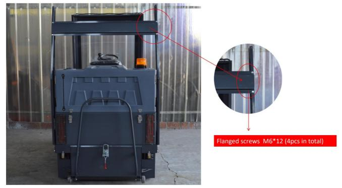
• STEP 4 Install the back mounting plate for the ceiling.
