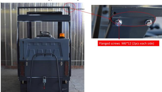
• STEP 5 Install connecting R-plate.
