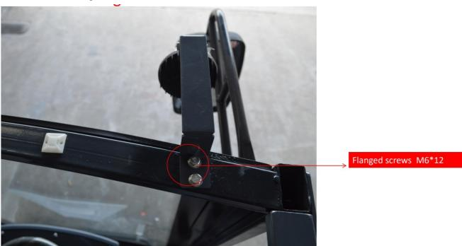
• STEP 8 Install the roof.
