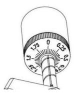
Rotate the counterweight counterclockwise (seen from the front) to adjust the downforce according to the cartridge manufacturer's recommendations. One mark on the scale represents 0.05g of downforce.
