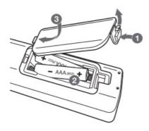
Remove the battery cover on the rear of the remote control, and insert the battery with + and – matched correctly. Risk of fire or explosion if the battery is replaced by an incorrect type.
