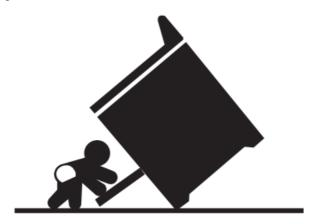
• Install the anti-tip device to the structure and/or the range. Verify the anti-tip device has been properly installed and engaged by following the guide on the anti-tip bracket template.
