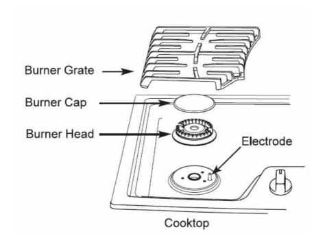
The burner head, the outer cap and the inner cap can be lifted off, making it easy to clean. The burner electrode is not removable.
