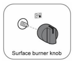
To reinstall a knob, hold it with the OFF label at the top and slide it directly onto the stem.
