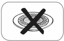
Do not use stove top grills on your surface burners. If you use a stove top grill on the surface burner, it will cause incomplete combustion and can result in exposure to carbon monoxide levels above allowable current standards. This can be hazardous to your health.
