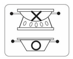
Flames larger than the bottom of the cookware will not result in faster heating of the cookware and could be hazardous.
