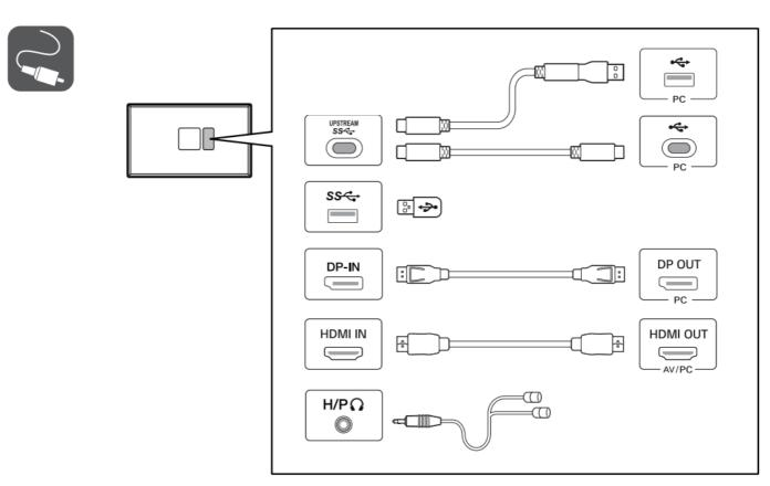
• Using a DVI to HDMI / DP (DisplayPort) to HDMI cable may cause compatibility issues.
