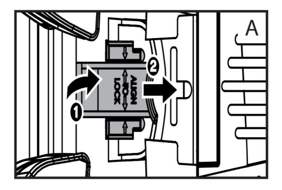
**STEP 1.** While looking inside the mask, move the locking clip rearward to the "unlocked position", by lifting up on the tab and pushing the Lock clip. (See Illustration A)
