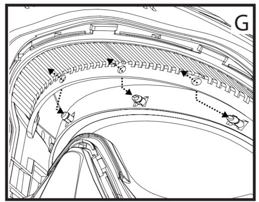
**STEP 1.** Holding the mask with one hand, firmly grasp the foam and plastic frame of the foam and pull away from the goggle.
