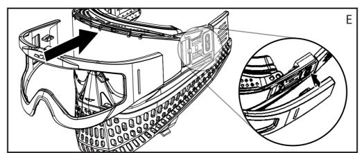
**STEP 3.** Holding the goggle in one hand, place the outer lens frame on the goggle, sandwiching the lens between the goggle and the outer lens frame. Make sure outer lens frame prongs glide smoothly into the goggle. (See Illustration E)
