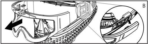
**STEP 3.** While holding the mask with one hand, grasp the side of the frame with your free hand exposing the outer frame prongs. Do the same for the opposite side and remove the outer frame from the goggle system. (See Illustration B)
