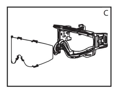
**STEP 4.** With the outer frame removed from the mask, the lens can be removed from the goggle. (See Illustration C)
