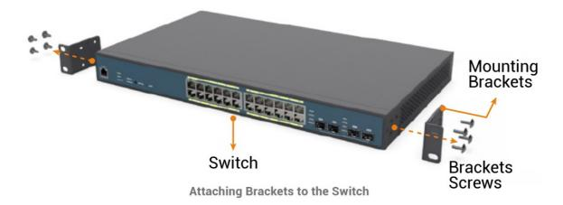
**Step 2**. Place the switch on a rack shelf in the rack. Push it in until the oval holes in the brackets align with the mounting holes in the rack posts.
