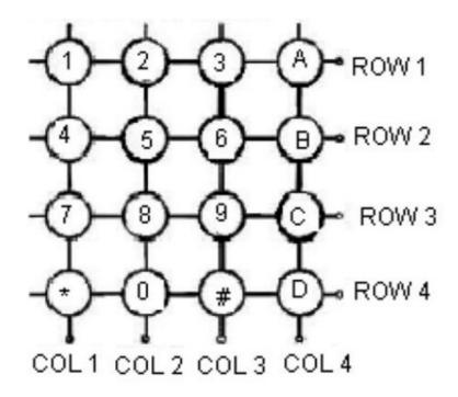
**Keypad with Arduino Circuit Schematic**
