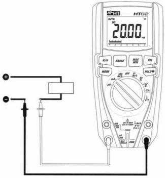
Fig. 10: Use of the instrument for DC current measurement
