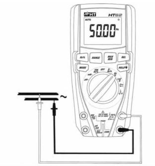
Fig. 5: Use of the instrument for frequency measurement and duty cycle test.
