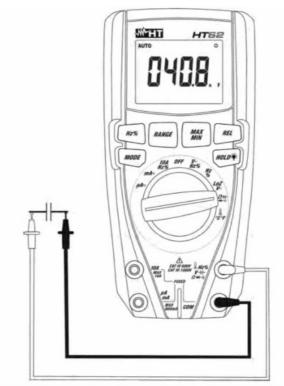
Fig. 8: Use of the instrument for Capacitance measurement
