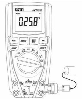
Fig. 9: Use of the instrument for Temperature measurement
