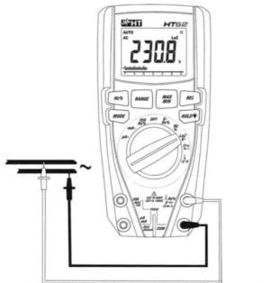
Fig. 4: Use of the instrument for AC/DC voltage measurement with low impedance (LoZ)
