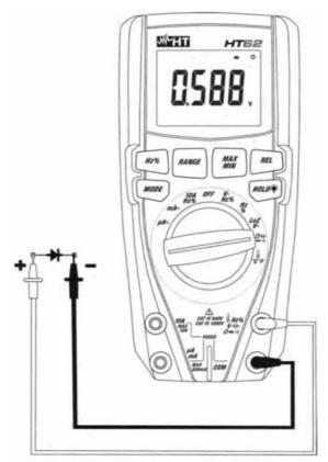
Fig. 7: Use of the instrument for diode test
