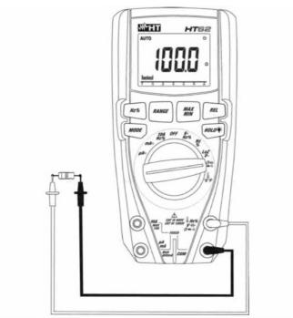
Fig. 6: Use of the instrument for resistance measurement and continuity test
