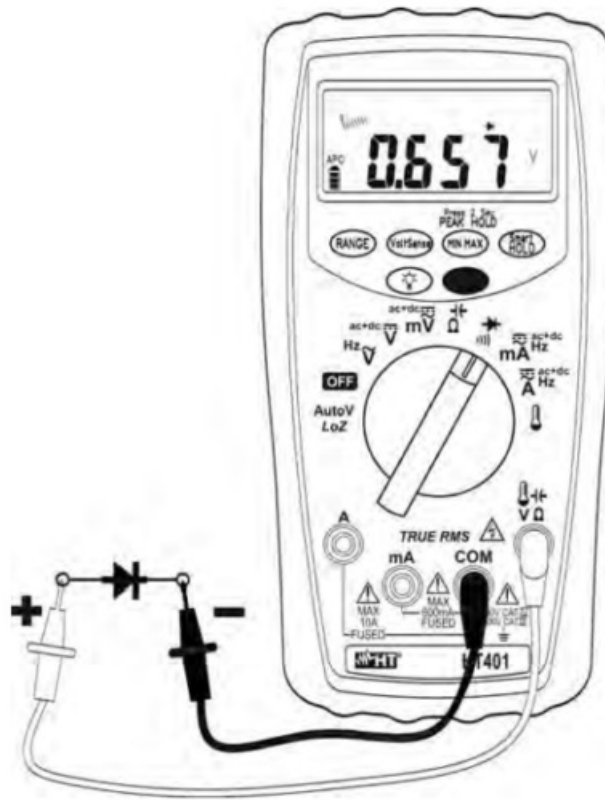
Fig. 8: Diode and continuity test
