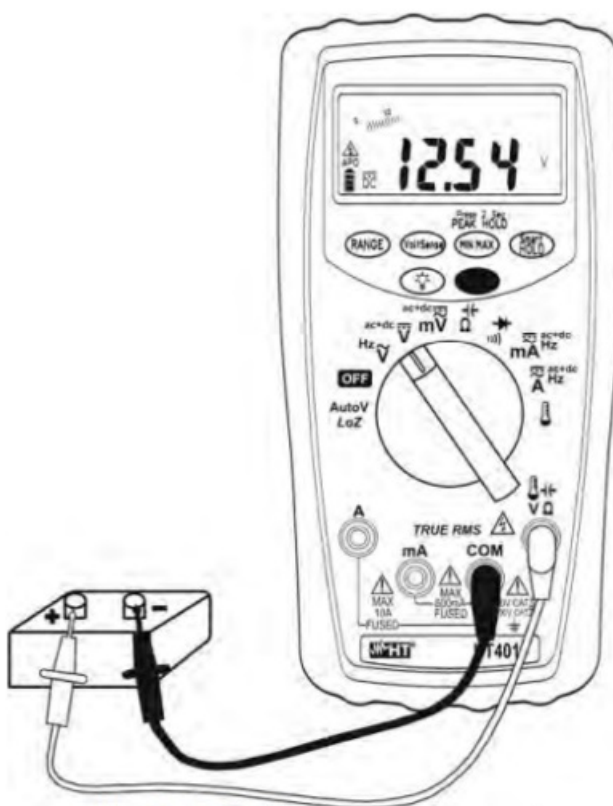
Fig. 2: DC voltage measurement
