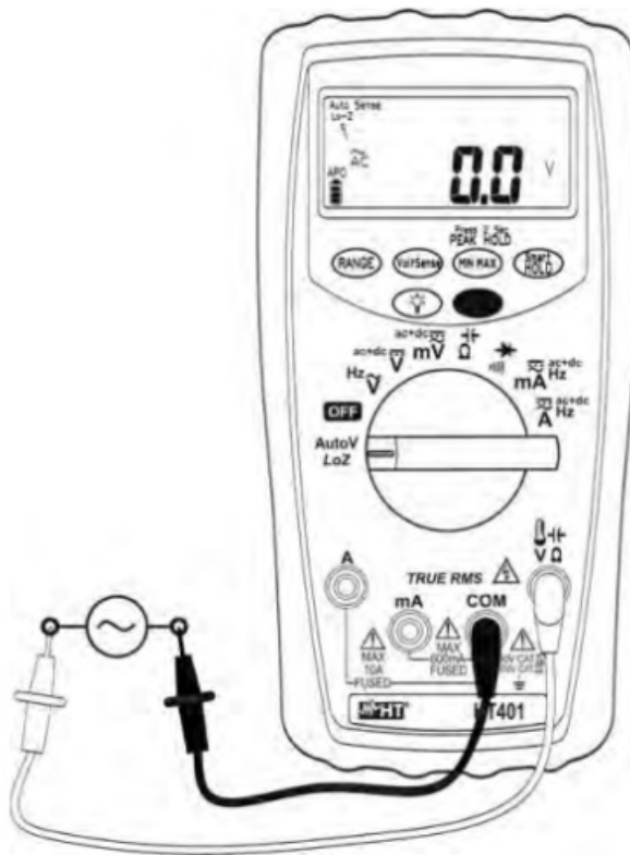
Fig. 4: AC voltage with low impedance (LoZ)
