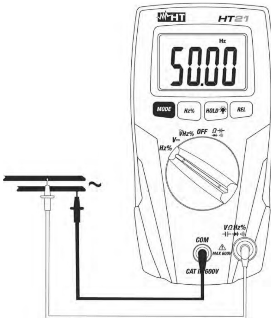
Fig. 3: Using the instrument for AC Voltage measurement
