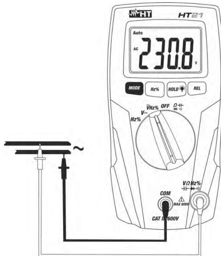
Fig. 6: Using the instrument for Frequency and Duty cycle measurements
