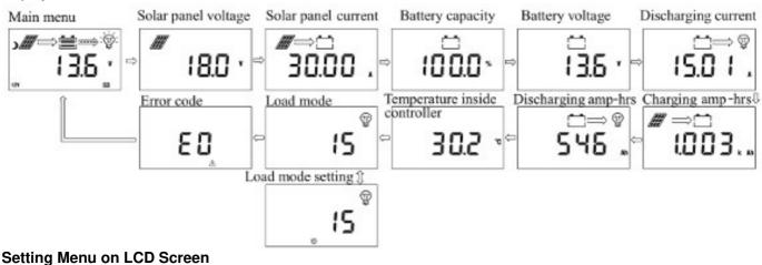
2). When "load mode" is displayed, long press to enter into the load mode setting. Press to adjust the mode, and long press for 2s to save and exit; or else, the system will not save the setting that was just made and automatically exit the setting interface after 12s.
