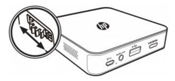
Adjust the focus by using the focus wheel on the left side to achieve a sharper image.
