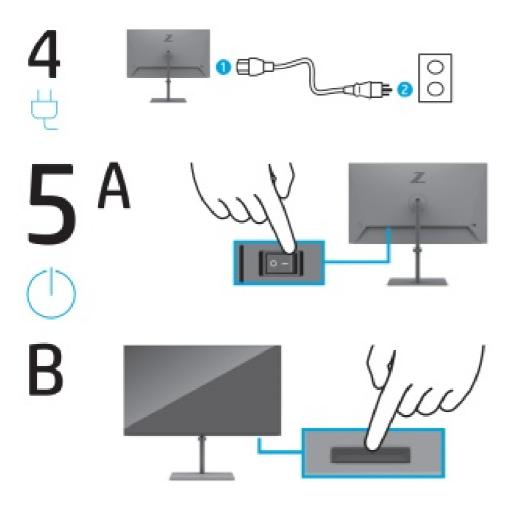
**WARNING:** To reduce the risk of electric shock, plug the power cord into an AC outlet that is easily accessible at all times. If the power cord has a 3-pin attachment plug, plug the cord into a grounded (earthed) 3-pin outlet.
