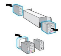
4. Insert each cartridge securely into the indicated slot. Close both doors.
