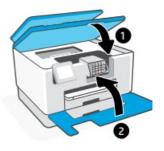
5. Open the paper tray. Slide out the front length guide, remove the cardboard, and slide out the width guides. Load a Letter or A4 paper and adjust the guides. Close the tray and pull open the output tray extender.
