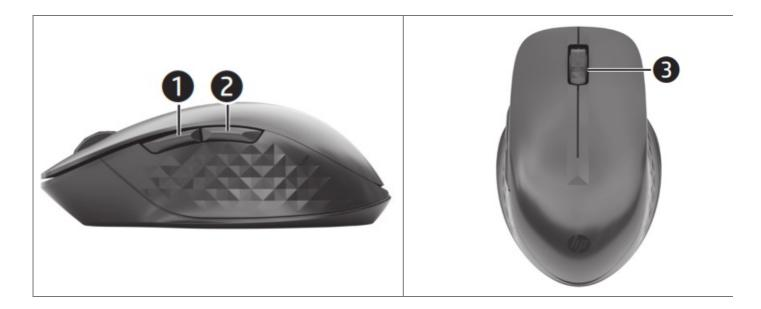
Connect the mouse to one computer using the receiver or one computer via Bluetooth®. To program the mouse buttons or change the DPI setting from 800 to 4000 DPI (default 1200 DPI), use the software. If the software does not download automatically, on your computer, open **Microsoft Store** or **Apple Store**. Search for **HP Accessory Center**, and then download the app.
