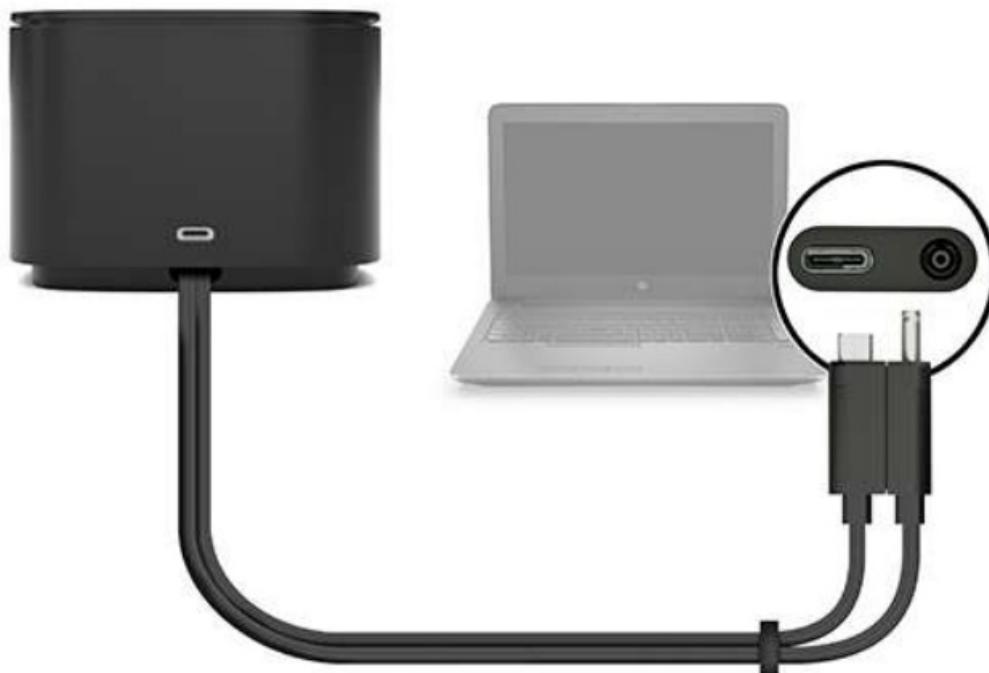
Figure 1-4 Connecting to a USB Type-C power connector and Thunderbolt port via the combo cable
