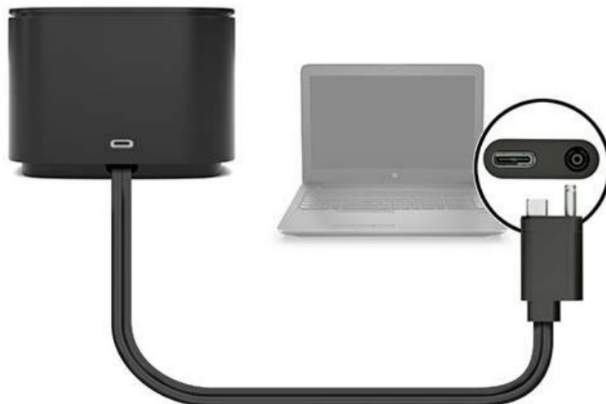
Figure 1-2 Connecting to a USB Type-C power connector and Thunderbolt port
