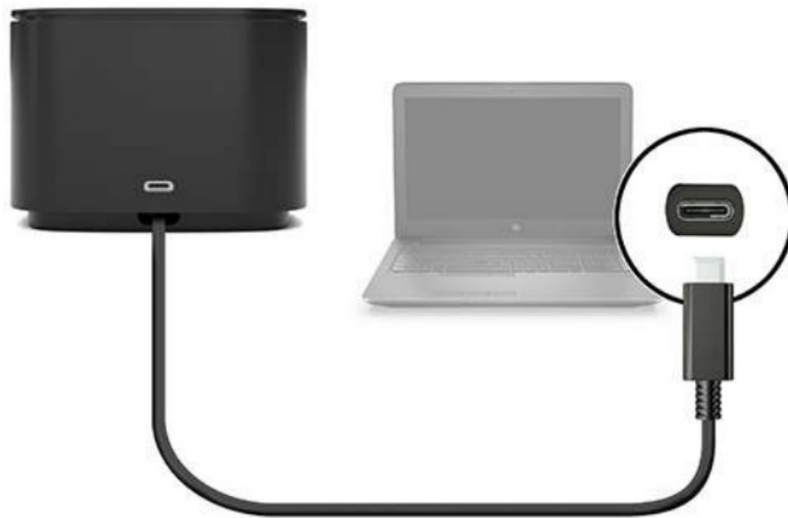
Figure 1-3 Connecting to a Thunderbolt port and power-in connector via the combo cable
