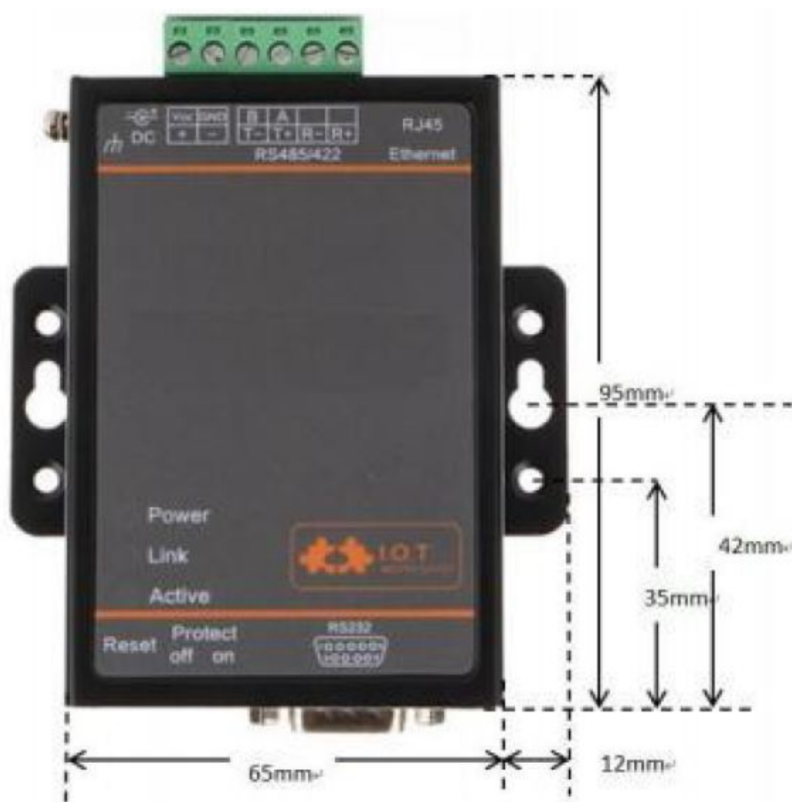
Figure 7. HF2211A Mechanical Dimension
