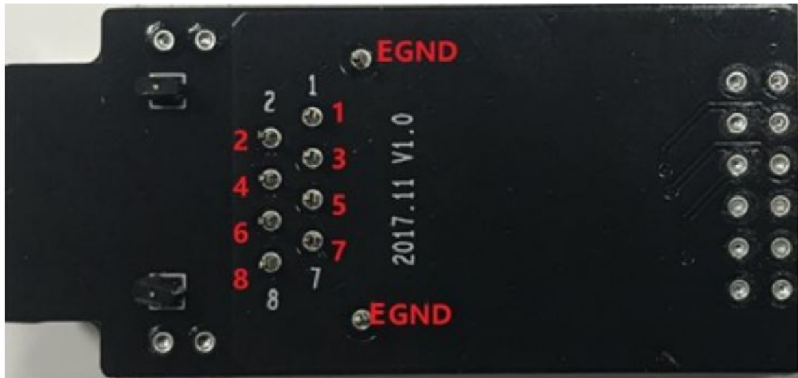
Figure 4. Eport-E20-PIN Pins Map
