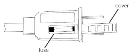
This plug contains an electrical fuse a safety feature.
