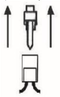
**Step 3:** Replace lamp with only 2.4 volt, 0.043 watt (Red/Amber yellow) or 3.8 volt, 0.068 watt (Blue/Green) LED type lamp (provided1 with product).
