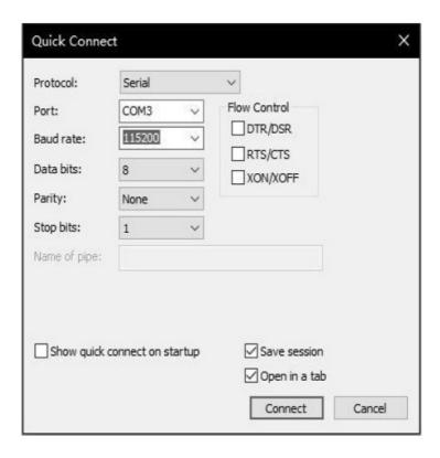
**NOTE:** COM Number can be viewed through device manager. (right click on my computer.>manage>device manager>port (COM and LPT). If it displays an unrecognized USB device, please download and install the corresponding driver.
