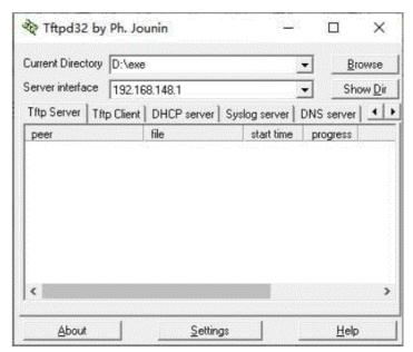
Open Tftpd32 software and set Server interfaces as the local IP address of the computer. Current Directory fills in the file path where the upgrade package is located. As the picture shows.
