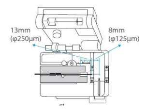
NOTE: Cut the bare fiber of 125µm to be 8mm with a cleaver and check the Length.
