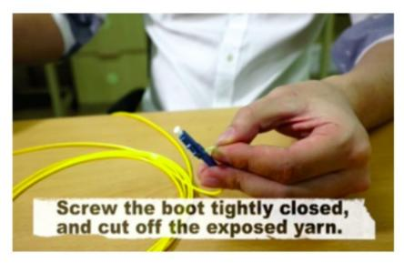
• To remove or re-terminate the connector, simple unscrew the boot and replace the jig
