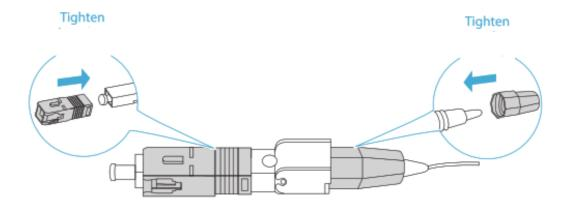
**NOTE:** Tighten the housing and the screw cap, then the fiber cannot be reassembled.
