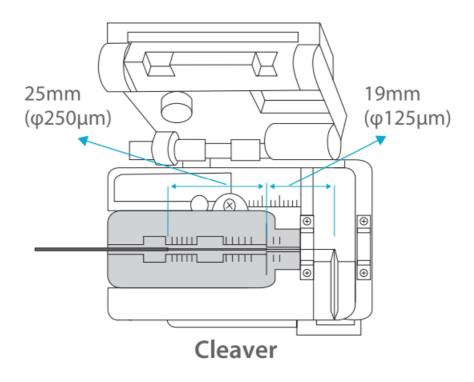
**NOTE:** Cut the bare fiber of  $125\mu m$  to be 19mm with a cleaver and check the length.
