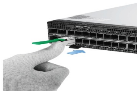
Figure 6: Latching the SFP-DD
