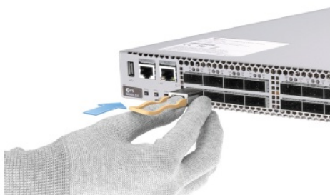
Figure 5: Latching the QSFP28
