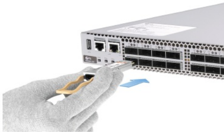
Figure 3: Inserting an 100G QSFP28 Transceiver Module into a Module Socket
