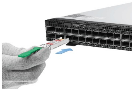
Figure 4: Inserting an 100G SFP-DD Transceiver Module into a Module Socket
