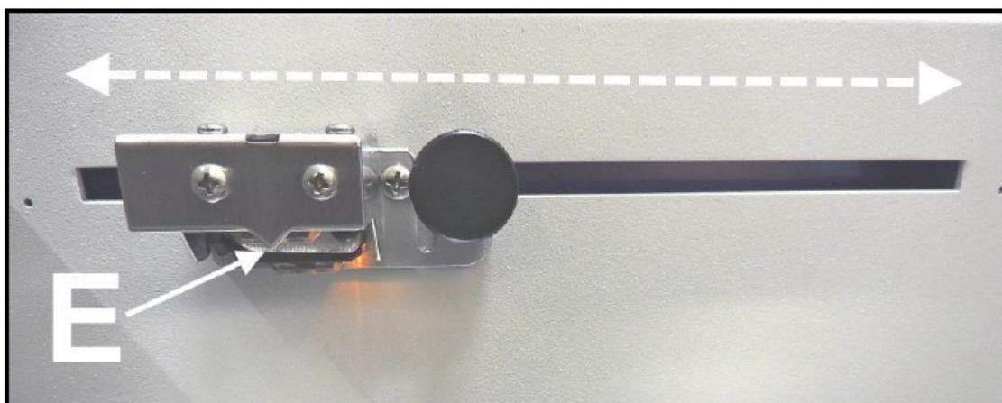
5. Adjust Rear Guide Support by using knob [F] to slide Guide right and left. If experiencing feeding problems, slide the Rear Support Guide right or left to keep media aligned with Media Guides.
