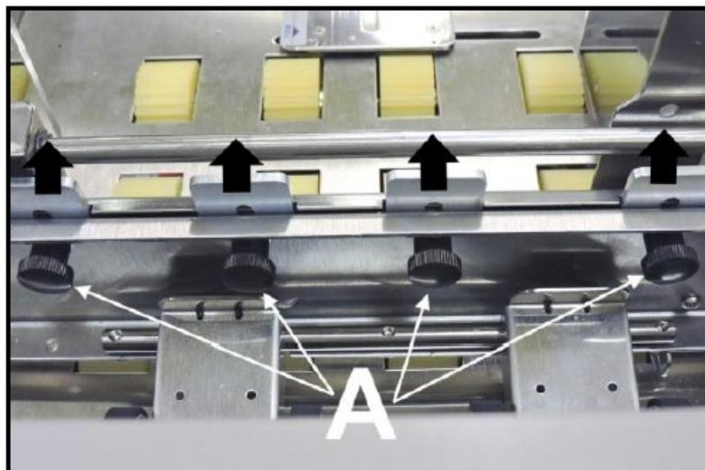
2. Place a single piece of media to be run under Separators. Always place media against Left-hand Media Guide [B]. Loosen Separator locking screw and allow Separator to settle onto media. Then tighten locking screw. Repeat for each Separator.
