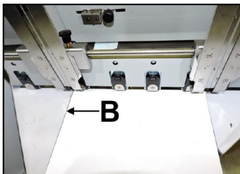
3. Position Adjustable Media Side Guide [C] so that it is about 1/32" from sides of media. Tighten locking knob on Side Guide [D]. Place a stack of media in machine. Press and hold Paper key to feed one piece through Separator. NOTE: To prevent misfeeds and tearing, keep the Adjustable Media Side Guide at least 1/8" from
