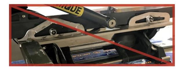
The photo above shows catastrophic damage to the Articulating Mechanism Channels from skiing NEXGen Fixed Outriggers without the U-Bolt.
