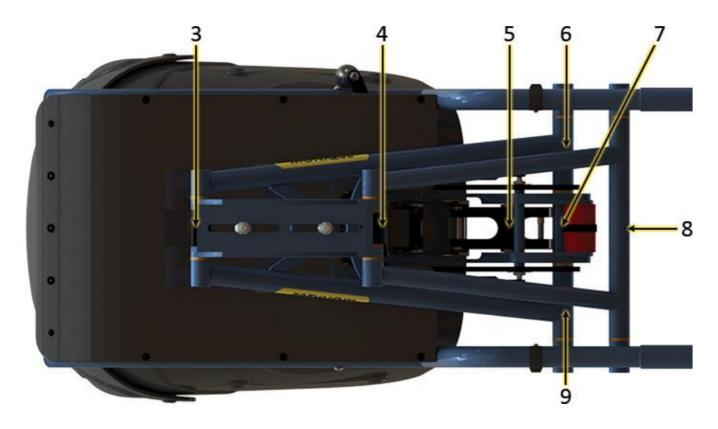
Lube the bronze bushing pivots with white lithium grease:
