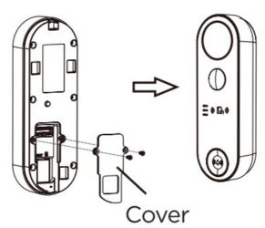
2. Attach the camera to the mounting plate using the lock screw (4x9mm) and L-wrench included with the camera.
