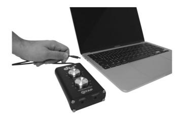
You can use a USB Type-C® to USB A adapter if your computer does not have a USB Type-C® port.
