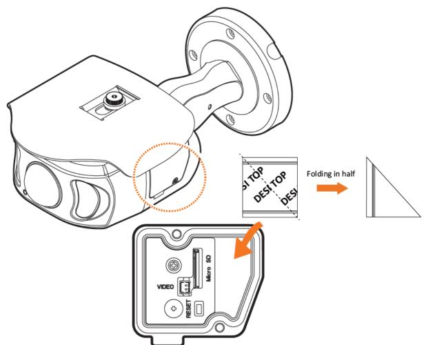
NOTE: The camera will generate enough heat to dry moisture during normal operation. In cases where the camera experiences a moisture issue, keep the moisture absorber in the camera.
