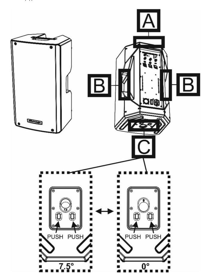
perfect for gigging bands as well as small venues installations. The 36 mm pole-mount predisposition is designed for use on a standard pole stand (like a tripod).
