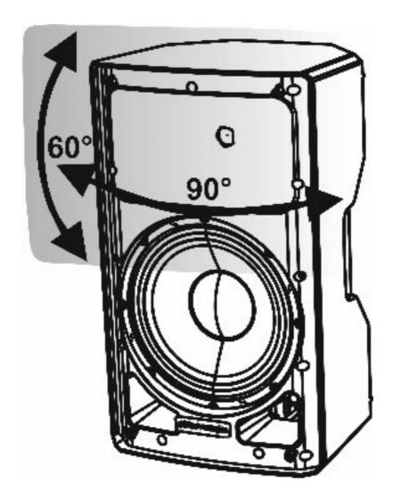
The acoustical design allows facing different environments. The dispersion pattern is shown in the upper picture. As described, the related pattern data are:
